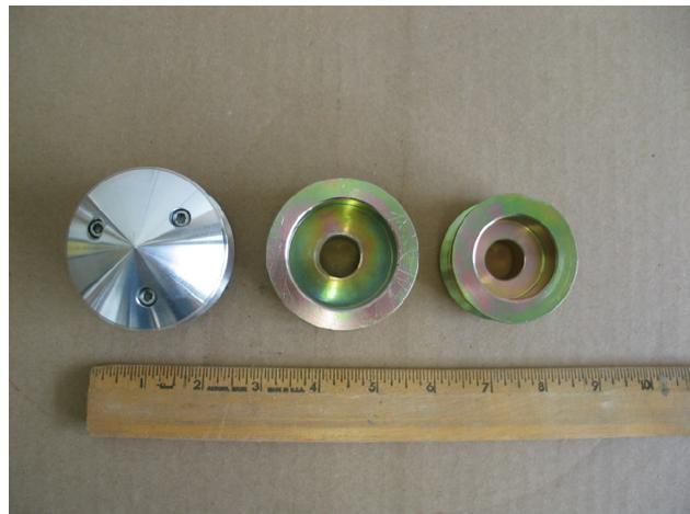
Now of course these are the stock steel pulleys which had 3 grooves on the crank and drove the water pump off of the power steering pulley instead of with the Alternator - a problem all by itself. I wanted to go to a serpentine belt and run the alternator off the same belt as the water pump while having a second position on the crank for an eventual air conditioning. The only way to get this done was to use a Ford small block kit by March Performance Pulleys - which utilized an under drive
