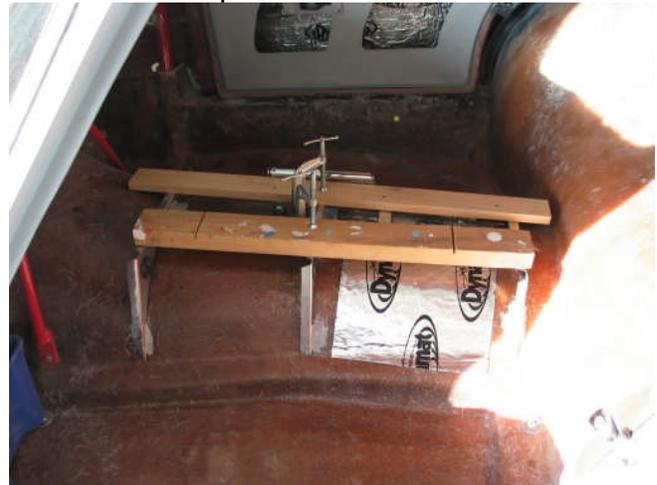
After letting the epoxy set up overnight I applied Dynamat Xtreme to the entire tunnel. The end result, less the dress panels, looks pretty good. Test fitting the seat shows I've got plenty of room along the tunnel for seat placement and it maintains a good top geometry, not too thin, not too wide.
