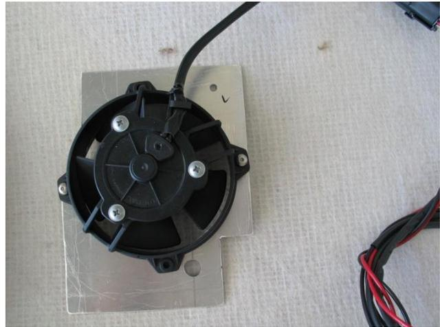
I found a suitable fan through a lot of searching and ordered two SPAL VA32-A-101-62A 12V fans which is a 4" fan, 2" tall and kicks about 240 CFM at about 3 amps each fan. They are used on ATV's and off road vehicles so they should survive inside my little heat box. Fabricating the bracket was simple with using foam core to get the basics and then transferring it over to .050" aluminum sheet.
