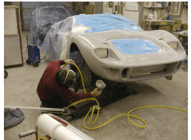
Ready for first primer coat Steve Karadi spraying first primer coat
