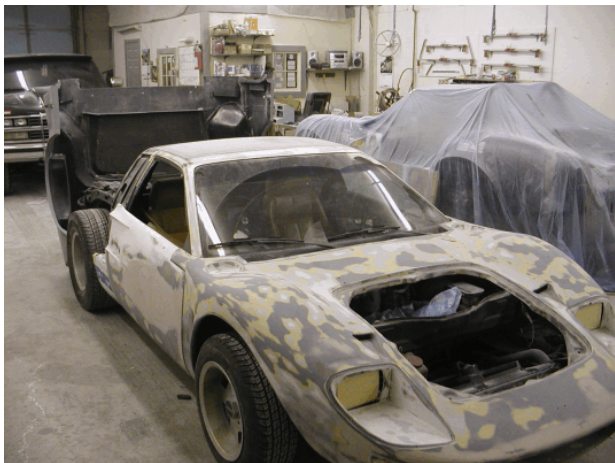
Ready for first primer coat Steve Karadi spraying first primer coat
